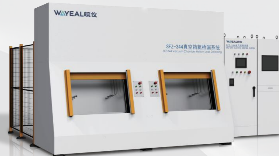
Manual Helium Detection Equipment for Automotive Parts
