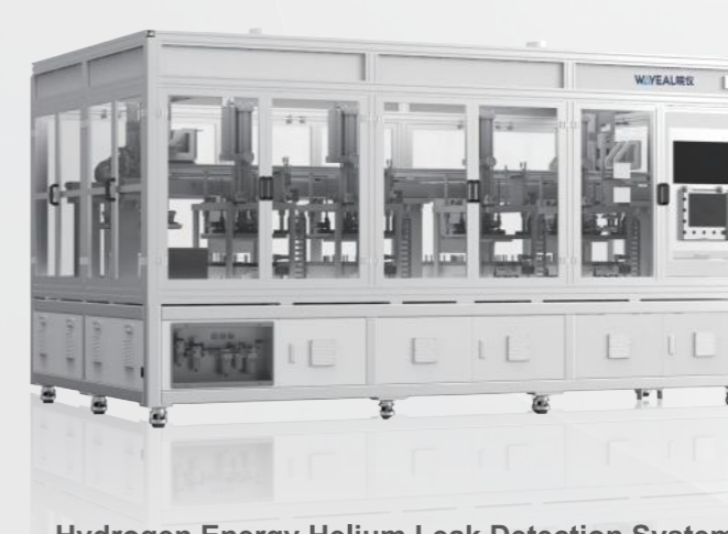
Hydrogen Energy Helium Leak Detection System
